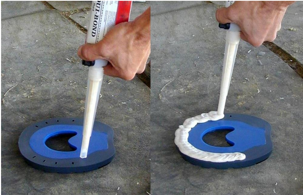
Figure 6: Use methacrylate adhesive, and be sure to put on enough.
