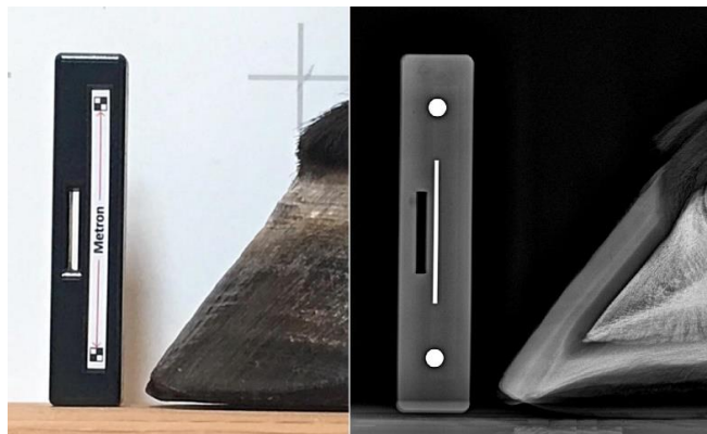
Figure 2: A two-ball scale marker. Left: photograph; Right: radiograph.
