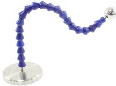
Figure 3: A one-ball scale marker (on a flexible positioner)
